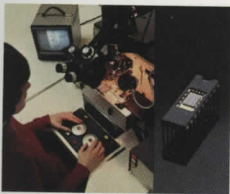
Microprocessor controlled bonding machines are used to complete the packaging of a device. A skilled operator performs the bonding operation once; the auto bonder remembers this "programming" and automatically bonds subsequent devices. The final packaged 2147, complete except for lid and final testing, is shown in the upper right.
