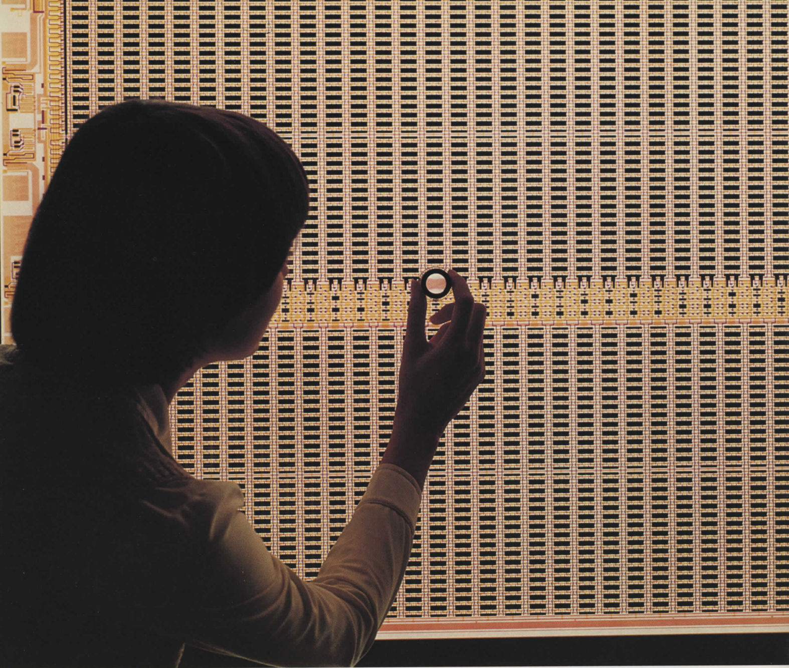
Individual masks, typically seven to ten levels, are utilized in the manufacture of MOS integrated circuits. The accuracy and registration of all levels is critical. Here they are checked at 200X final size.
