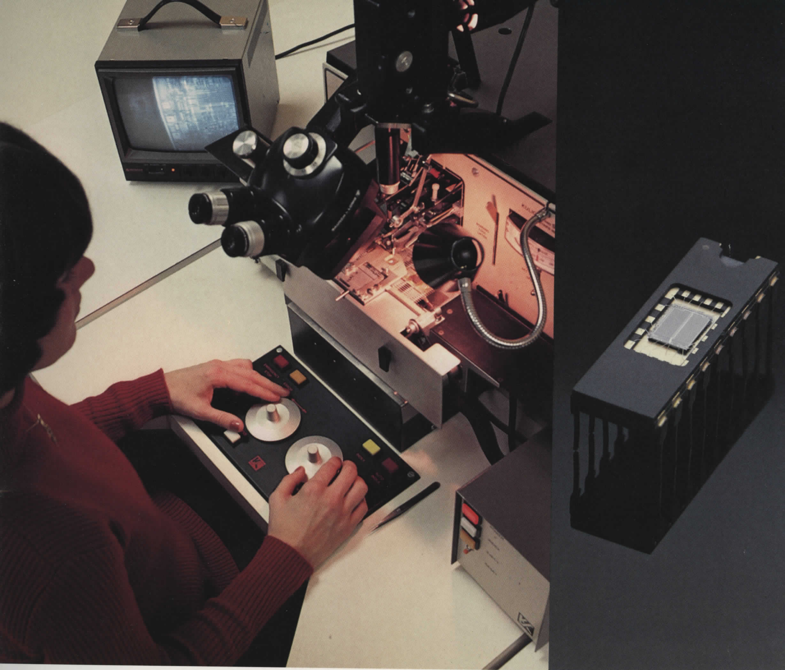
Microprocessor controlled bonding machines are used to complete the packaging of a device. A skilled operator performs the bonding operation once; the auto bonder remembers this "programming" and automatically bonds subsequent devices. The final packaged 2147, complete except for lid and final testing, is shown in the upper right.
