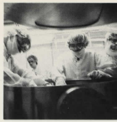
Routine equipment maintenance is critical to fab productivity. Equipment engineering services technicians work on a sputtering system, Fab VI.
